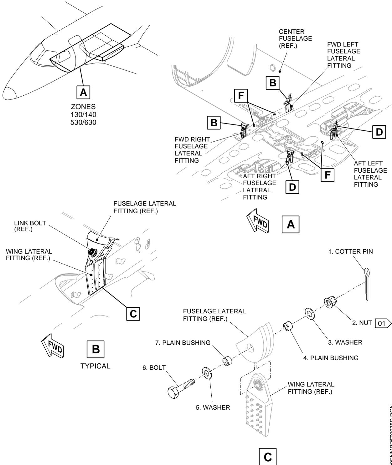
**01** DRAG TORQUE: 5.65 – 45.2 N.m (50 – 400 lb.in) ADDITIONAL TORQUE: 56.5 – 214.7 N.m (500 – 1900 lb.in).
